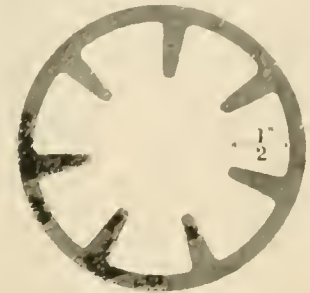
SERVE TUBE, 2 1/2 INS. OUTSIDE DIAMETER, SHOWING INTERNAL PROJECTIONS.
